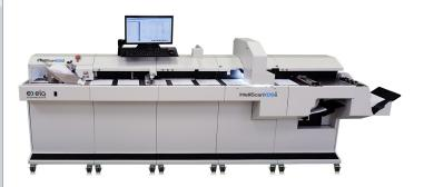
With a completely open track, the IntelliScan XDS<sup>5</sup> offers the least restrictive paper path in its class, simplifying document retrieval in the rare event of a paper jam. The IntelliScan XDS<sup>5</sup> also features the error recovery module which increases document throughput by allowing quicker recovery from problems, minimizes the number of documents to be re-fed and reduces the chances of missing or out-of-sequence documents.
